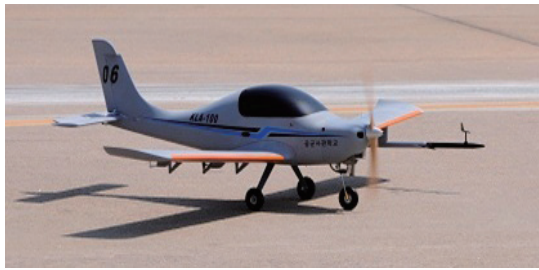
Fig. 17. Scaled RC-model of KLA-100 for flight tests
