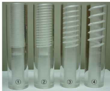
Fig. 3. Helical grain configurations
