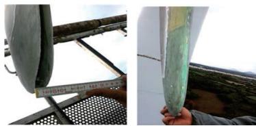
Fig. 1. Damaged and repair tip blade of wind turbine [9].
