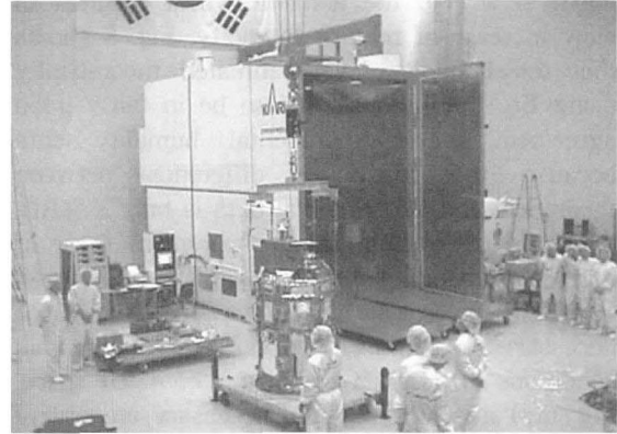
Fig. 3. The overall view of a large-sized thermal humidity chamber and KOMPSAT-1 PFM located in front of the chamber
