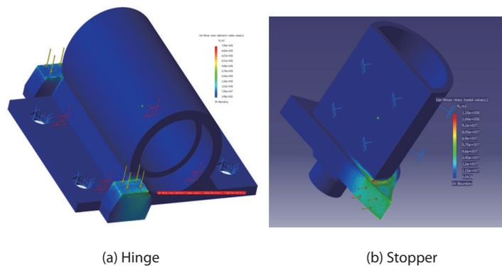
Fig. 11. Von-Mises stress distributions of hinge and stopper
