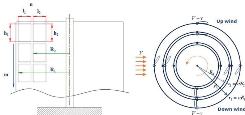
Fig. 2. Arrangement of split flapping blades with upward splits m by outward splits n
