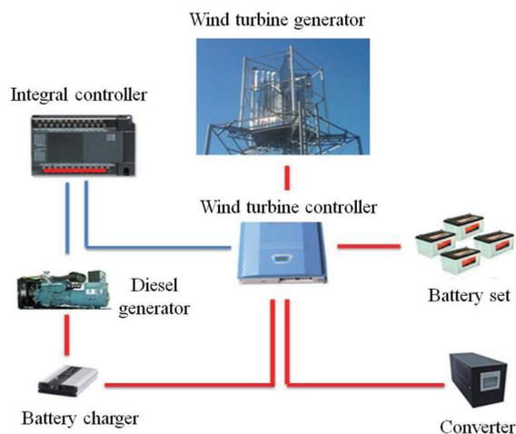
Fig. 13. Hybrid electric power generation system
