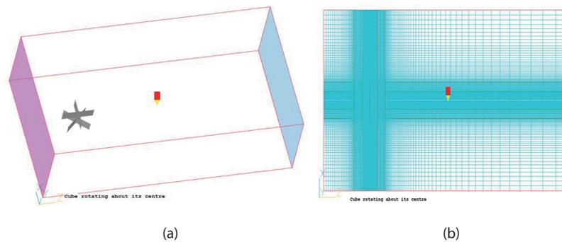
Fig. 6. Perspective view of wind turbine model (a) and 3-D numerical analysis mesh generation of wind turbine model (b)
