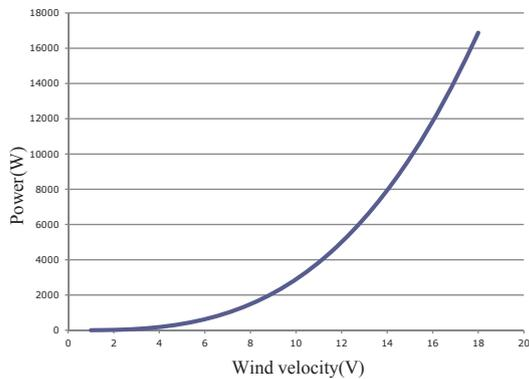
Fig. 5. Estimated power of the 2x5 split case wind turbine
