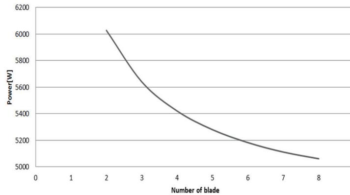
Fig. 3. Power versus number of inward split blades (upward split is fixed as 2)
