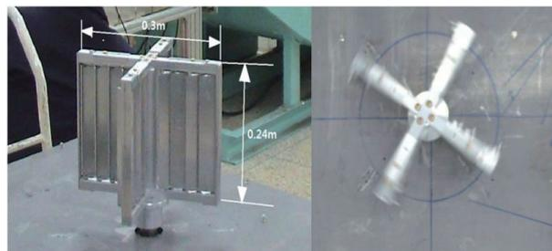
Fig. 10. Subscale model of the flapping wind turbine blade assembly
