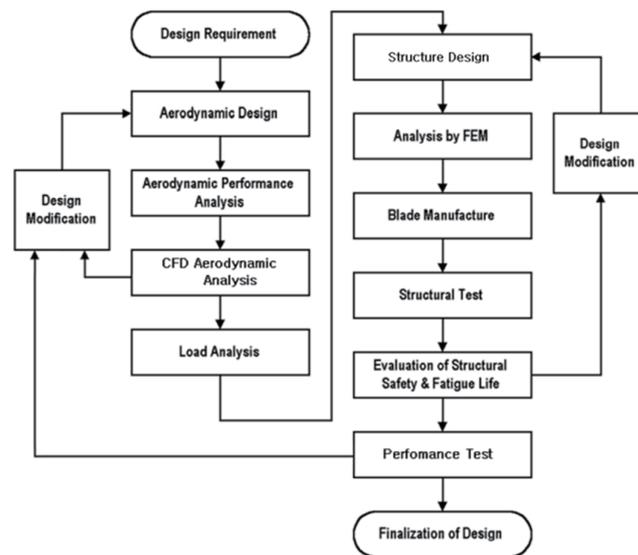
Fig. 1. Proposed aerodynamic and structural design Procedure
