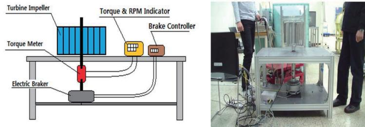
Fig. 9. Schematic view and picture of subscale wind turbine model performance test setup
