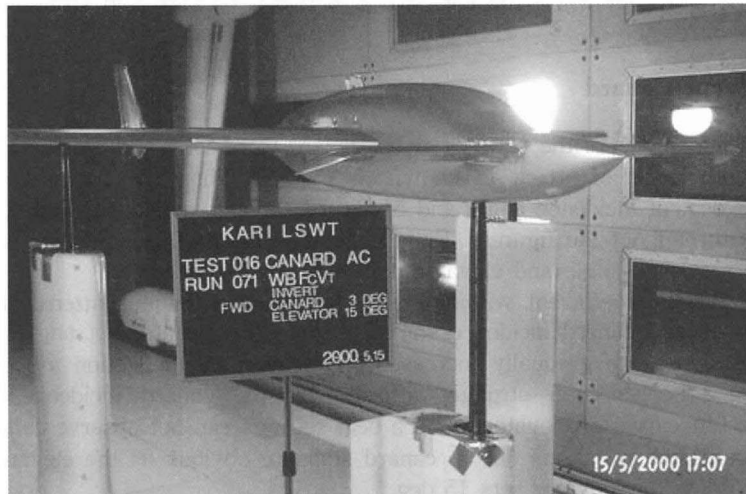
Fig. 2. Canard model in Test Section
