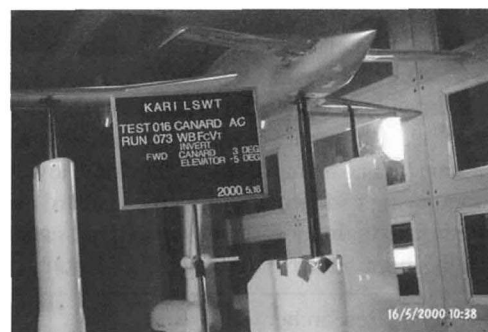
Fig. 1. Straight(left) and Forward Swept Canards
