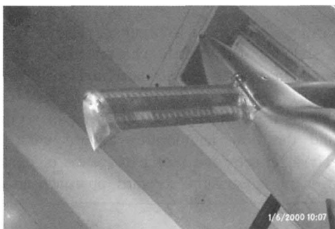
Fig. 1. Straight(left) and Forward Swept Canards
