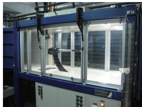
Fig. 3. Closed-circuit wind-tunnel test section with sting balance
