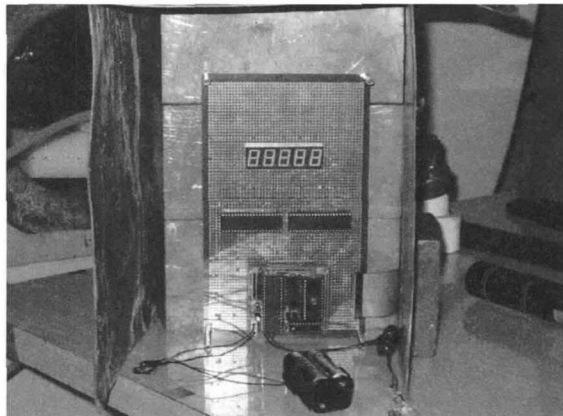
Fig. 3. The testing controller board surrounded by plumbum (Pb) blocks at the Cyclotron accelerator
