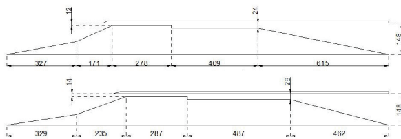
Fig. 2. Conceptual design of RBCC propulsion system [2]
