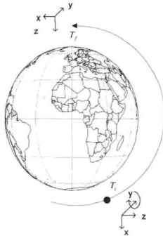
Fig. 8. Maneuver to the nadir-pointing from sun-pointing
