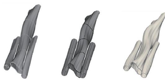
(a)  $f_{3D} = 11.63$  Hz (b)  $f_{2D-1D} = 13.78$  Hz (c)  $f_{LE} = 13.98$  Hz
