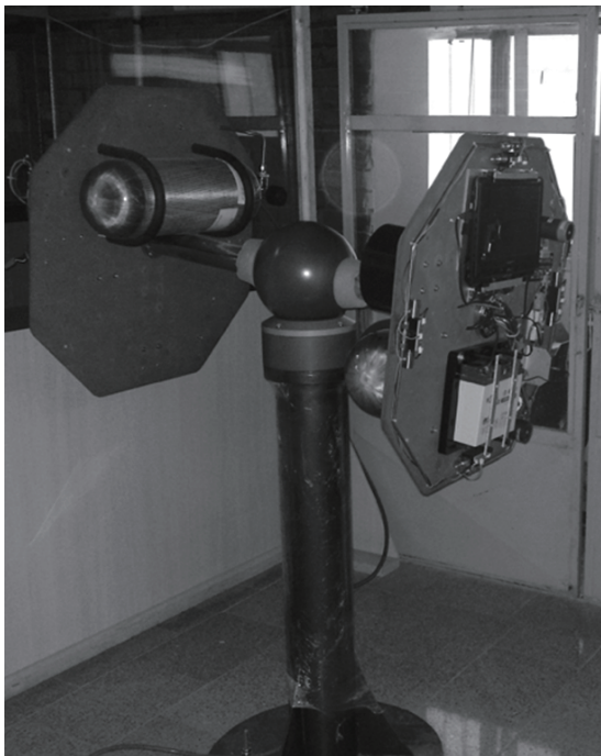
Fig. 6. The attitude control simulator in Space Research Laboratory
